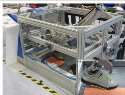
Fig. 1: TUM TrakTester (modified to measure longitudinal bending stiffness in athletic footwear)
